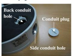
4. Disconnect the power and video wire from the camera board end of the wire. Gently pull the wire out from under the plate until it is free. Using wrench or pliers, remove the weather tight bushing from the rear conduit hole. Using the plug removed in step 3 above, close the rear conduit hole (additional caulk or other sealant recommended).
